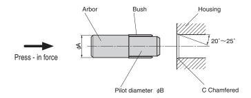
Arbor dia =Housing I.D.– $(0.2 \sim 0.4 \text{ mm})$
